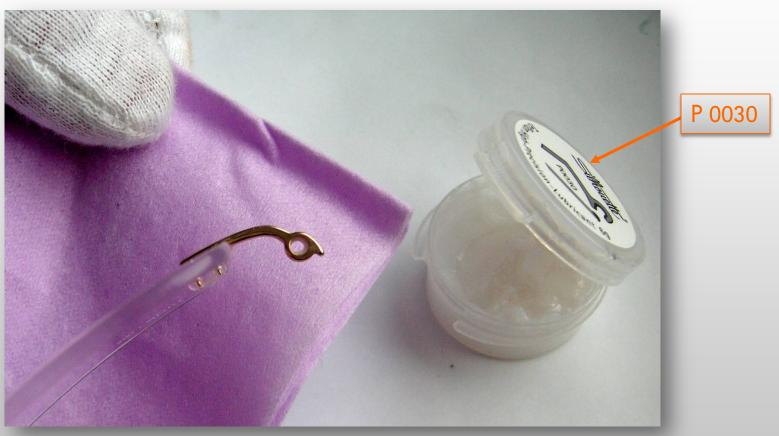
Grease the inside loop of hinge with high precision lubricant (P 0030). If necessary clean beforehand. Mount small plastic part. Assemble temple.
