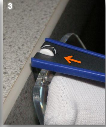
1. Place temple exactly at the slot of the BLShinge 2. Push hinge against protected table edge as far as possible into the temple.
